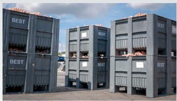
Safe hold: Integrated locking devices (stacking cams), on the four corners of the CB3 box ensure safe stacking. Photo: Craemer Group
