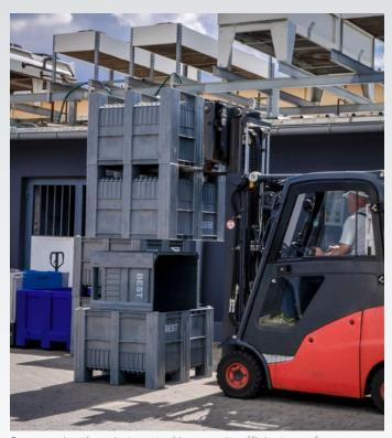
Space-saving three-in-two stacking permits efficient use of space during empty transport and storage Photo: Craemer Group
